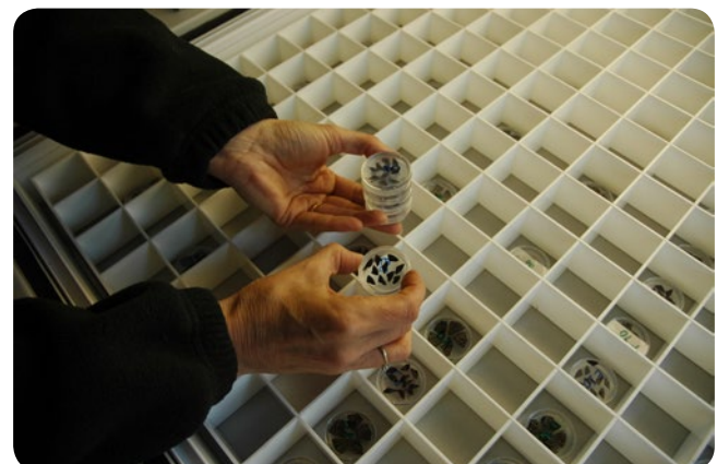
Temperature gradient plate used to investigate temperature thresholds for seed germination, with inset of individual temperature cells.
