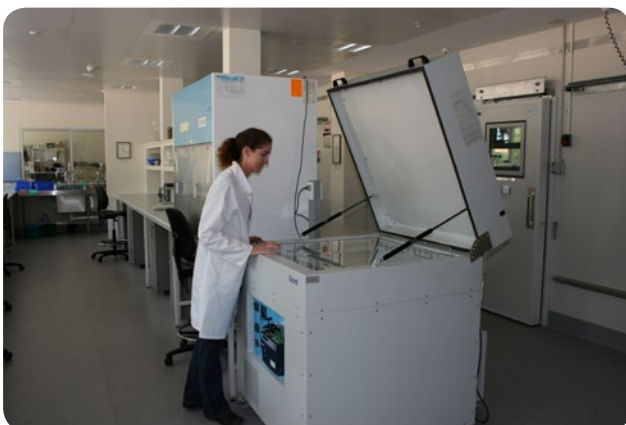
Temperature gradient plate used to investigate temperature thresholds for seed germination, with inset of individual temperature cells.
