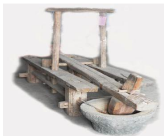
Chedui (a kind of stone mortar): also called "duichong", used for hulling rice.
