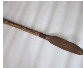
Pizai (a knife with two edges and a short wooden handle): also called “double edged Qindao”, used to clear the weed on the ridges and walls.
