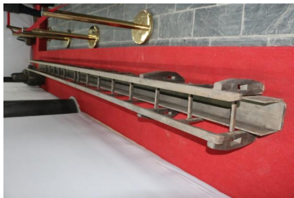
Figure 1-3-25 Dragon-bone waterwheel in Ziquejie and Hakka Terraces
