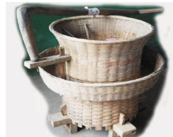
Tulong: also called "leizi", a tool made of bamboo strip for removing rice peel
