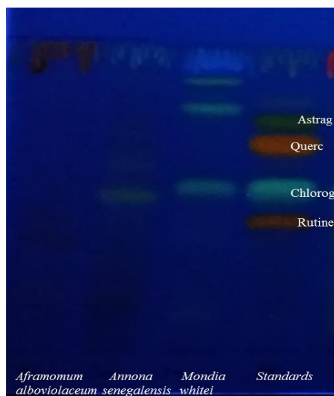
Figure 6a. TLC Chromatogram of methanolic extracts of studied plants using controls at 366 nm
