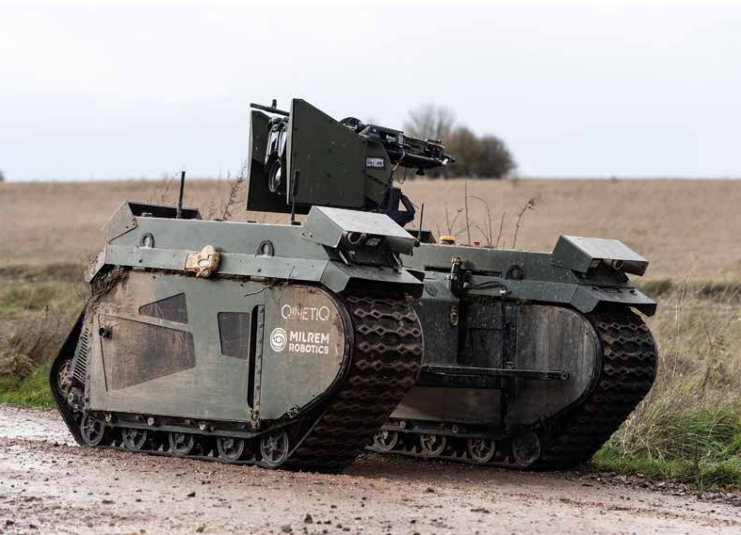
Pictured is the QinetiQ Titan Strike, a large tracked UGV with a laser rangefinder system and fitted with a machine gun undergoing tests in the toughest of simulated combat environments at Copehill Down training facility near Chitterne during Exercise AUTONOMOUS WARRIOR. Photo: Corporal Rebecca Brown, Crown Copyright
