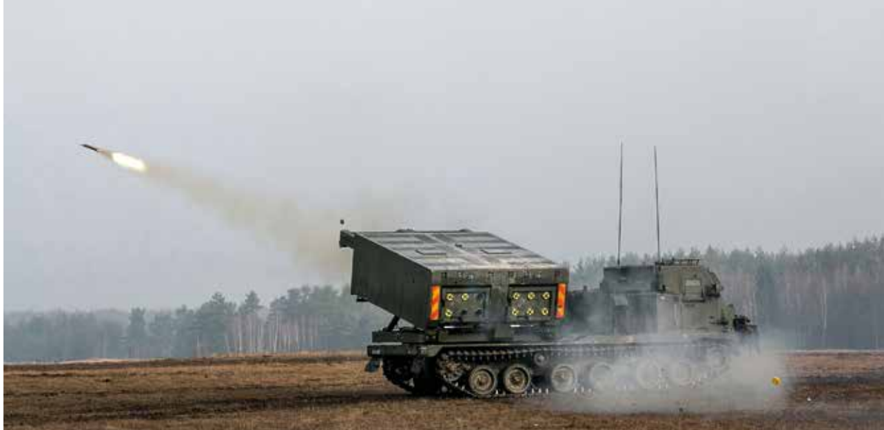
British soldiers from 176th Battery, 19th Regiment Royal Artillery, conduct live fire training using the Guided Multiple Launch Rocket System (GMLRS) during Dynamic Front 18 in Grafenwoehr in Germany. Photo: Specialist Dustin Biven, Released
