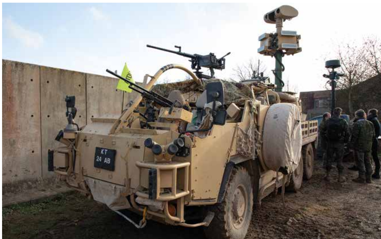
Pictured is M-AUDS, a mobile Counter UAV detection system mounted on the back of an in-service Coyote platform which can identify, classify, track and defeat UAV's. Unmanned Aerial Vehicles and Unmanned Ground Vehicles will be trialled to measure how they can support surveillance, resupply, command and mobility. Photo Sergeant Peter George, Crown Copyright.
