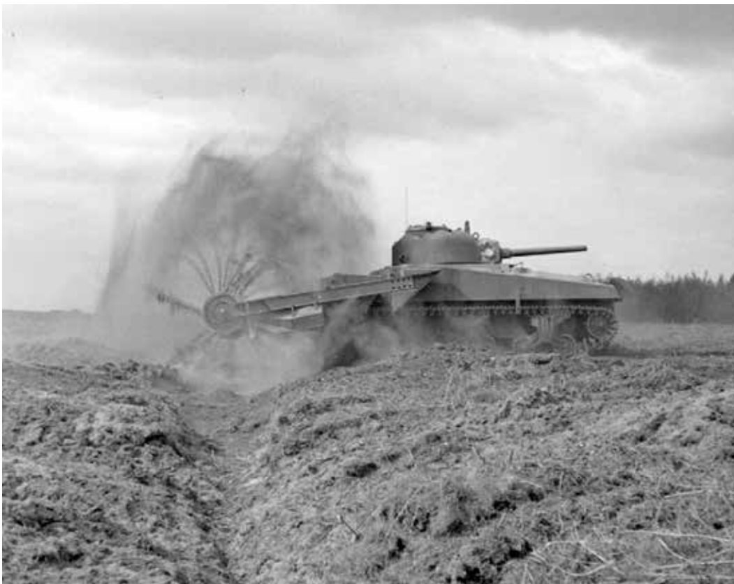
Sherman crab flail tank under test, 79th Armoured Division. Copyright IWM H38080, Wikimedia.
