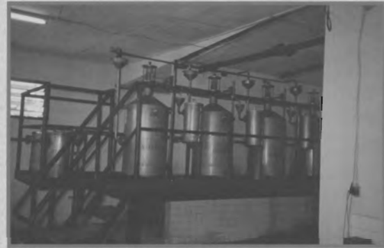
Figure 1.7 A modern Cajuput oil distillation facility at Krai in Central Java: (top left) four of the eight 0.9 tonne capacity pots at the facility; (bottom left) the steam boiler which is fuelled entirely by leaves and twigs dried after distillation; (right) stainless steel separators for collecting the oil.
