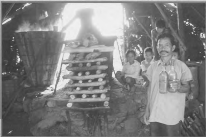
Figure 1.5 M. cajuputi oil production on Buru Island is a family concern: (top) this producer air dries M. cajuputi leaves in the sun before distillation; (bottom) a basic wood-fired still and condenser made of wood and mild brass. Wood for the fire is stacked for drying in front of the fire. The producer is holding bottles of Cajuput oil ready for sale.
