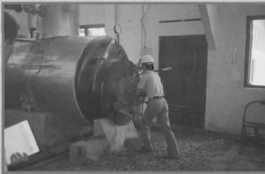
Figure 1.7 A modern Cajuput oil distillation facility at Krai in Central Java: (top left) four of the eight 0.9 tonne capacity pots at the facility; (bottom left) the steam boiler which is fuelled entirely by leaves and twigs dried after distillation; (right) stainless steel separators for collecting the oil.
