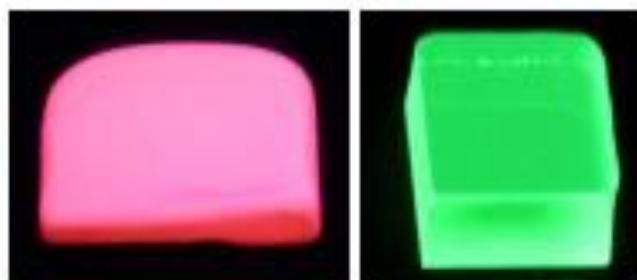
Demonstrates the luminescence emission colors of willemite based glass-ceramics by excitation with a weak UV lamp at 254 nm which can be used for various applications
