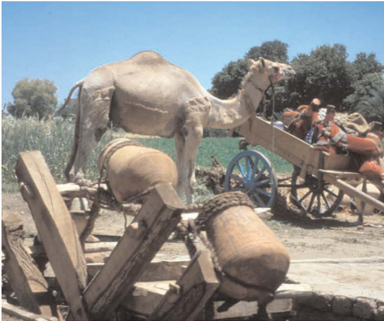
Rotating wheels and cogs help dip clay jugs into an underground water source.
