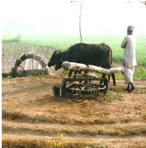
An oxen-drawn cog draws water out of a well and spills it into an adjacent irrigation channel.
