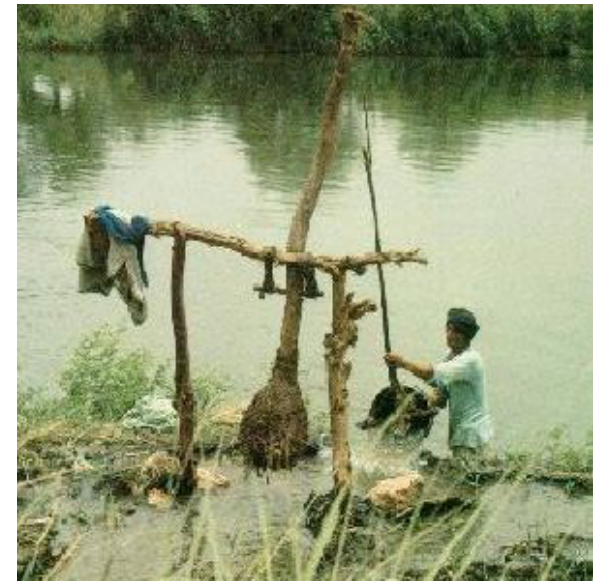
Drawing water up from the river to irrigation channels with a shadoof in Egypt.
