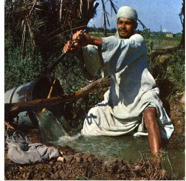
Pumping water from a lower to an upper terrace with an Archimedes screw in Egypt.
