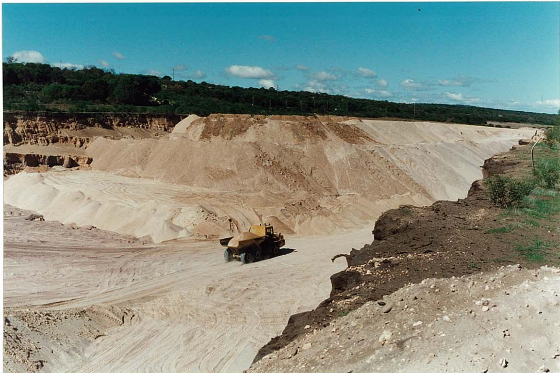
View looking South - East over the backfill dump. Overburden and tailings are used to backfill the pit as it moves northward, recreating a natural looking topography.
