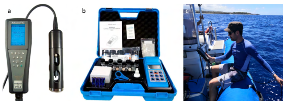
Figure 16: YSI Quatro +© multiparameter probe (a), Hanna instruments TUB430© field turbidimeter (b), in situ deployment (c) (MAREX, 2023)
