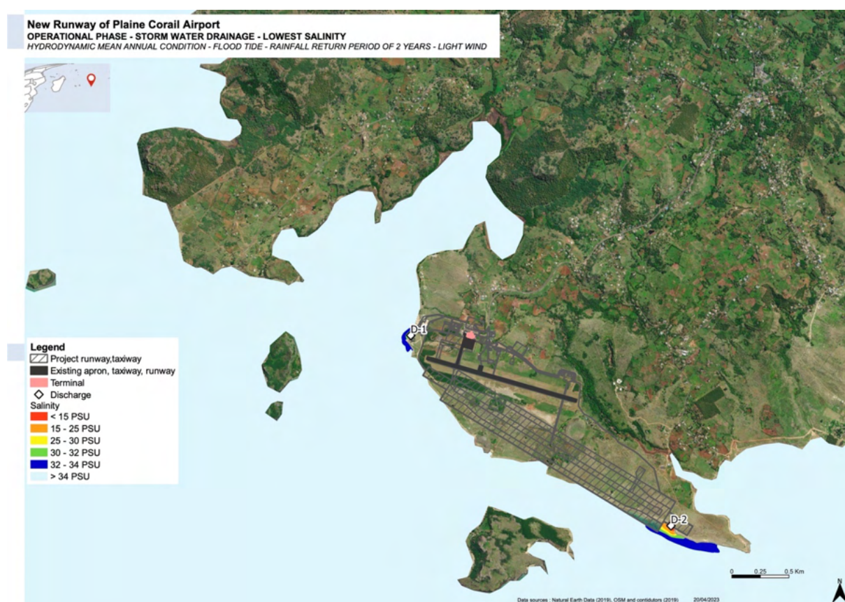
Figure 32: Stormwater drainage plumes model (SETEC, 2023)
