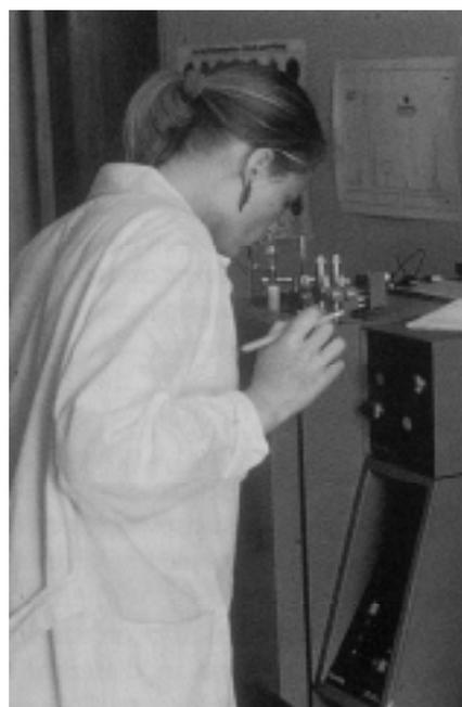
**Fig. 2.** Gas chromatograph equipped with headspace and sniffing detector.
