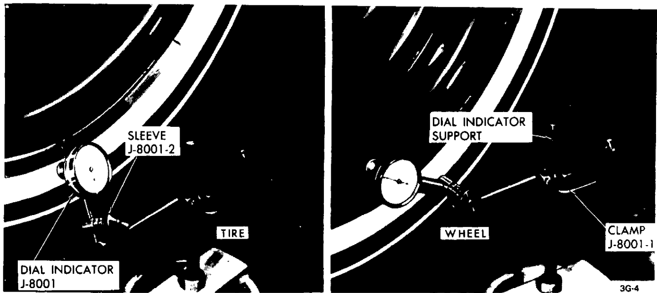
Figure 3G-4 Checking Lateral Runout
