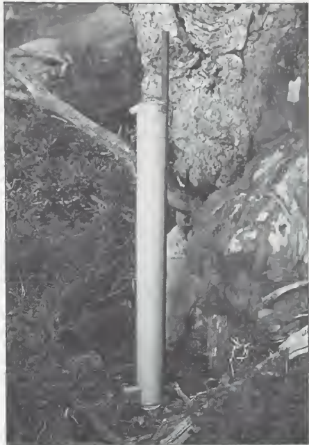
Fig. 1. View of the pipe erected to allow pitfall traps to be extracted through the snow without disturbing the snow cover. The pitfall can be seen in the gap at the bottom of the pipe.
