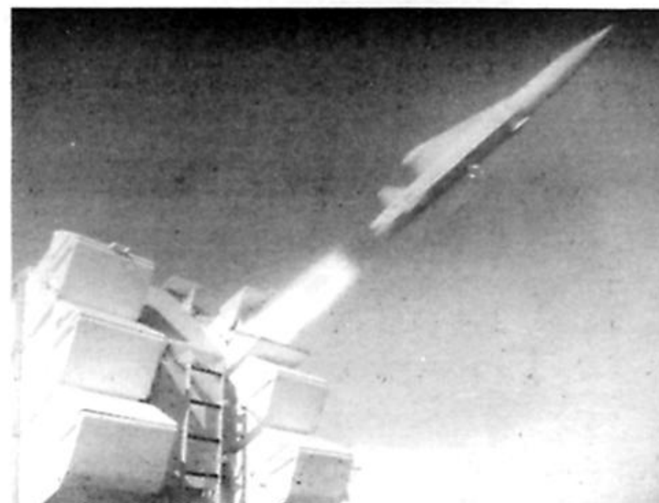
H.M.S. Broadsword fires her Sea Wolf air defence missiles for the first time. The all-missile frigate, currently in the midst of long and exacting first of class trials, brought her Sea Wolf launchers into action off Halifax, Nova Scotia. Each launcher comprises two groups of three barrels mounted on a trainable frame.
