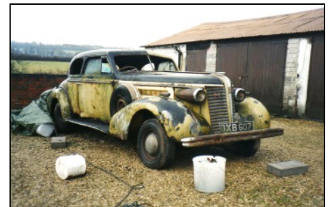
1937 Buick Convertible Coupe before restoration, a hardtop from another car had been welded on
