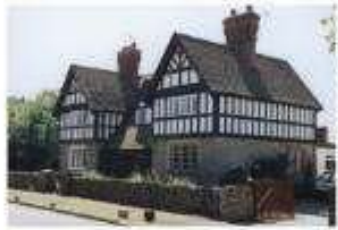
Great Alne Hall (since 1876) was apparently of similar style to the West Lodge and Packardside and Rosemary Cottages (left), which are built in the Victorian "mock-Tudor" style with rubble stone ground storey and timber-framed first floor gables.
