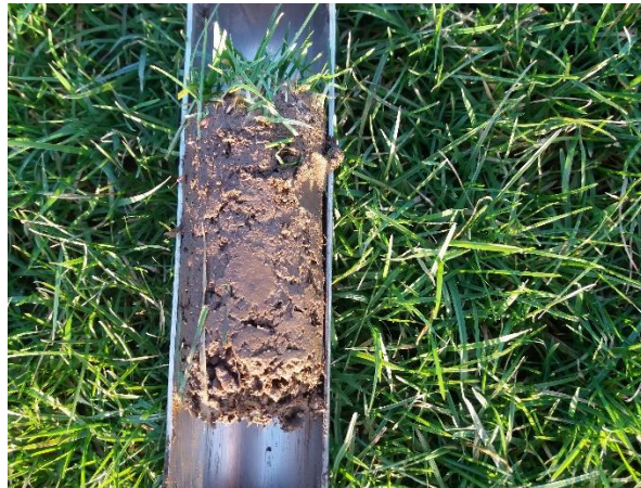
Figure 4: Heavy soils dominate the site and are more prone to deformation following heavy rainfall. Additional drainage would enhance long term performance and playability.
