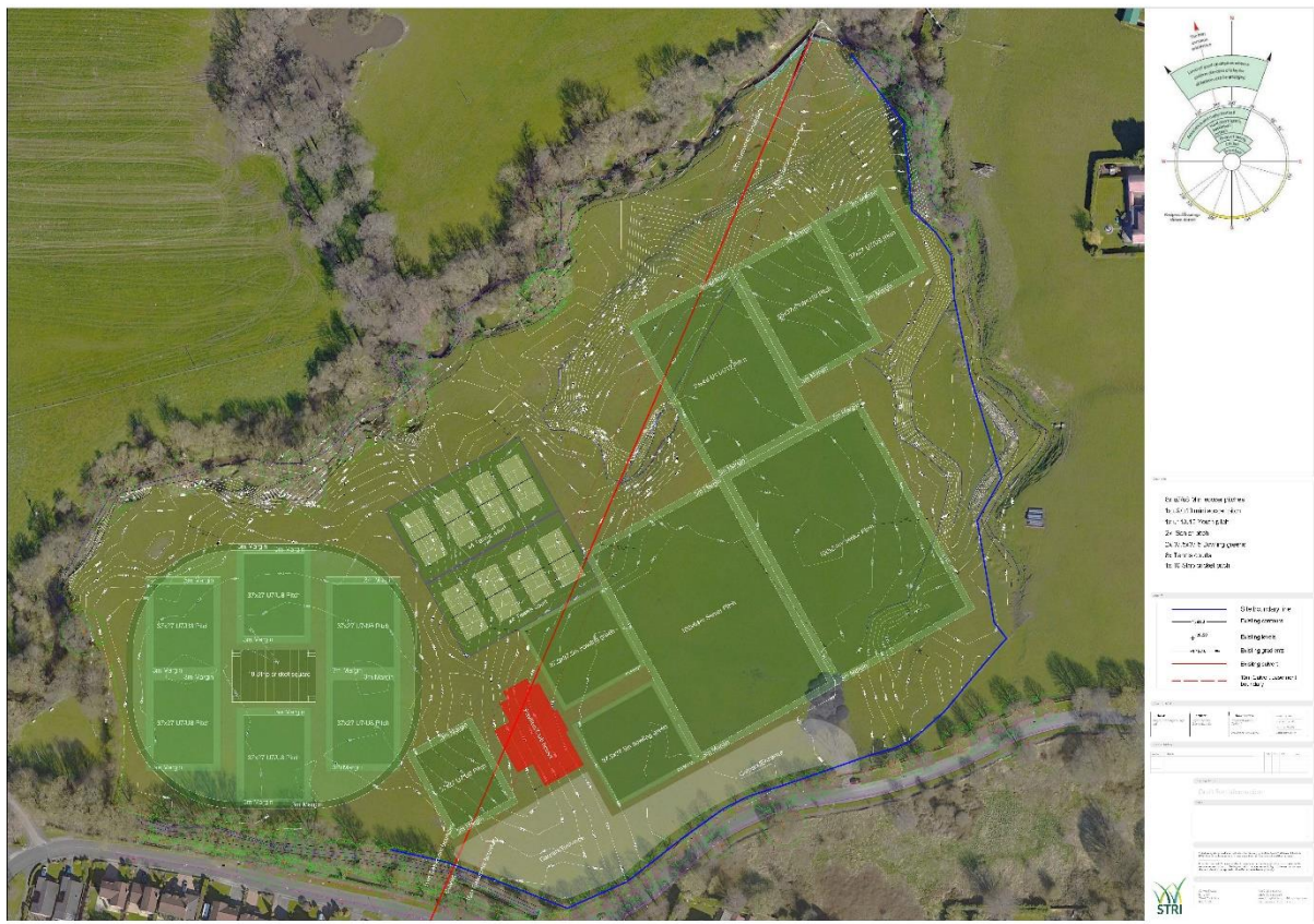
Figure 1: Layout of STRI proposed sports pitches. Pipeline traversing the site is shown by the red line.
