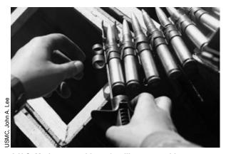
A U.S. Marine assembles .50-caliber ammunition onto a link belt, 2002.
