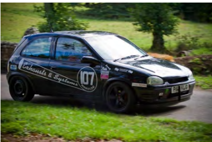
Vauxhall Development Car 1400cc – 1800cc conversion producing 182 BHP @ wheels, new developments for 2016
