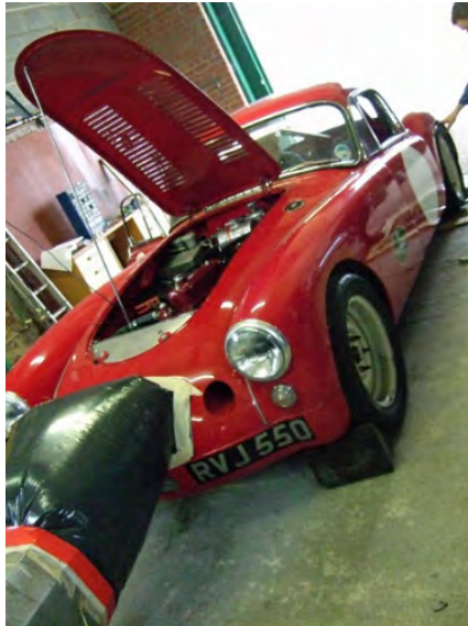
Vauxhall Development Car 1400cc – 1800cc conversion producing 182 BHP @ wheels, new developments for 2016
