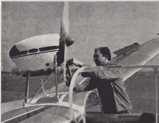
◀ Shown on left, the JAWA 42-h.p. motor unit mounted on Blanik.
