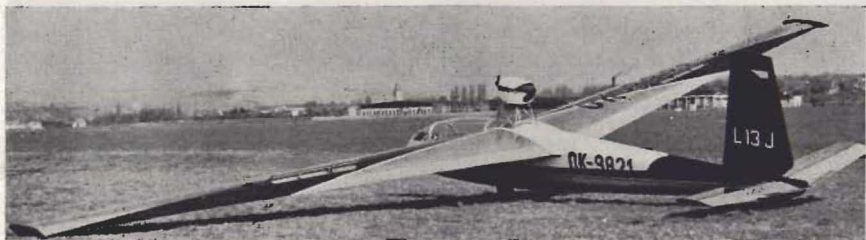
▲ The Blanik with detachable engine pod.
