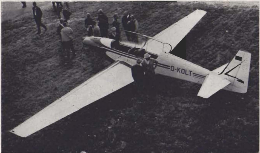
▼ The two-seater RF-5 with Volkswagen engine.
