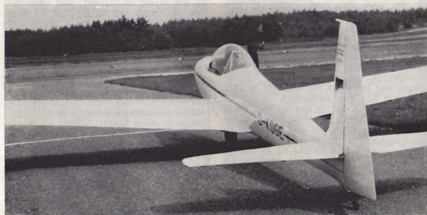
The SF-27M, engine retracted. (Photographs by P. Jeffers)
