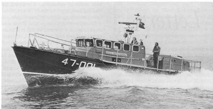
(above) City of London, the first 47ft fast slipway lifeboat prototype, at sea. Her operational trials, just started, must of necessity be long and exacting, but she is already showing herself to be sea-kindly, dry and of an encouraging speed.
