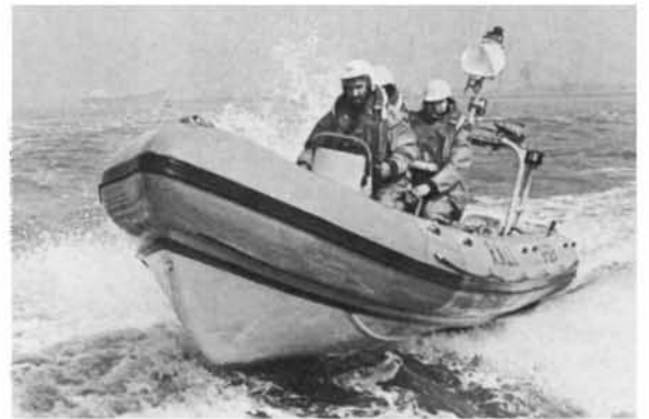
(above) Atlantic 21: length overall 22ft 6in; beam 7ft 6in; draught, including engines, 2ft 6in; displacement 1 ton; maximum speed, 29 knots; range at full speed, 70 nautical miles. The Atlantic 21, introduced in 1972, has a crew of three and launches from a carriage. Her hull is GRP with an inflated neoprene sponson. photograph by courtesy of Keith Yuill Photographic
