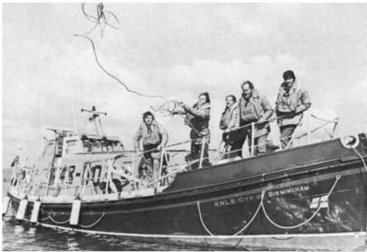
(left) Solent: length overall, 48ft 6in; beam 14ft; draught 4ft 6in; displacement 27 tons; maximum speed, over 9 knots; range at full speed, 240 nautical miles. The Solent, introduced in 1969, is a development of the 48ft 6in Oakley and she has a crew of seven; she launches down a slipway or lies afloat. Her hull is built of steel. photograph by courtesy of 'Birmingham Post and Mail'
