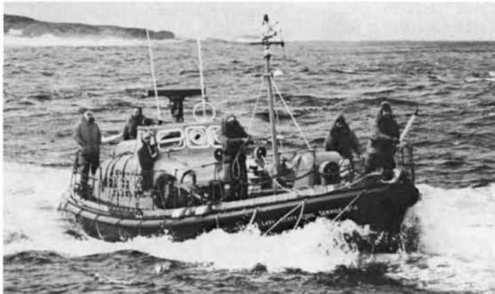
(above) Rother: Length overall 37ft 6in; beam 11ft 6in; draught 3ft 6in; displacement 13 tons; maximum speed, 8 knots; range at full speed, 150 nautical miles. The Rother, introduced in 1973, is a development of the 37ft Oakley and she has a crew of seven; she launches down a slipway or from a carriage, or she can lie afloat. Her hull is built of wood.
