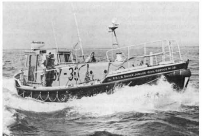
(above) Rother: Length overall 37ft 6in; beam 11ft 6in; draught 3ft 6in; displacement 13 tons; maximum speed, 8 knots; range at full speed, 150 nautical miles. The Rother, introduced in 1973, is a development of the 37ft Oakley and she has a crew of seven; she launches down a slipway or from a carriage, or she can lie afloat. Her hull is built of wood.
