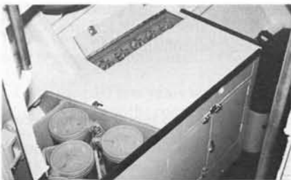
(below) . . . and the worktop lifts up to give access to Speedline line throwing apparatus and its igniters (top centre).
