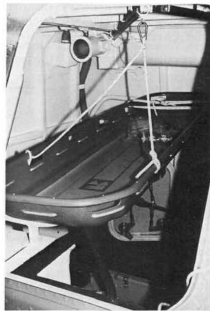
(below) There are permanent positions for two basket stretchers in the after cabin, one to starboard and one to port. Note trackway to which a steadying bridle can be attached when lowering stretcher-borne injured survivors into the resting position.
