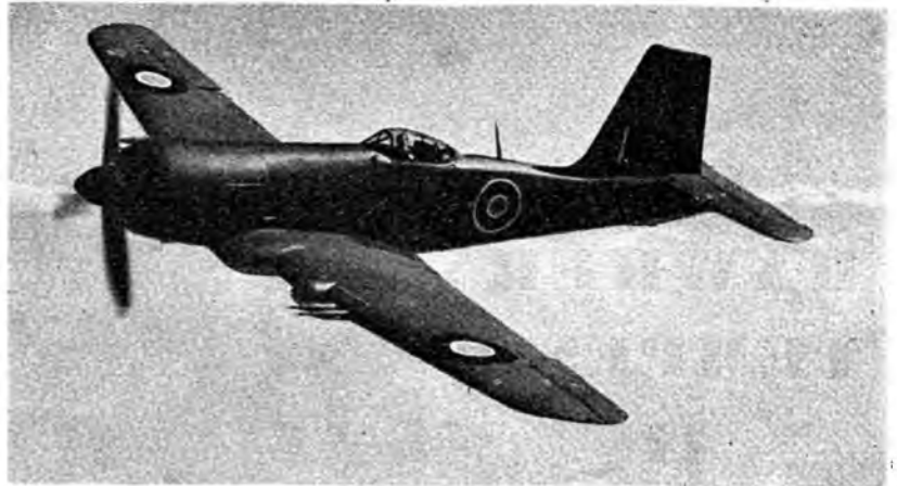
Best Brand Blackburn —This Firebrand IV is one of the most formidable of the new generation of "strike" aircraft for the Royal Navy, and can function as a torpedo-bomber, dive-bomber, rocket-fighter or normal fighter. Blackburn Photo.
