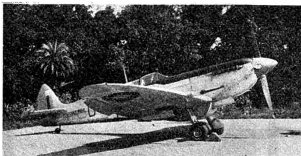
Shining Armour. —First picture to be published of a Spitfire fighter in natural aluminium finish, with black anti-dazzle cowling. This particular aircraft is a Spitfire VIII of South-East Asia Command.
