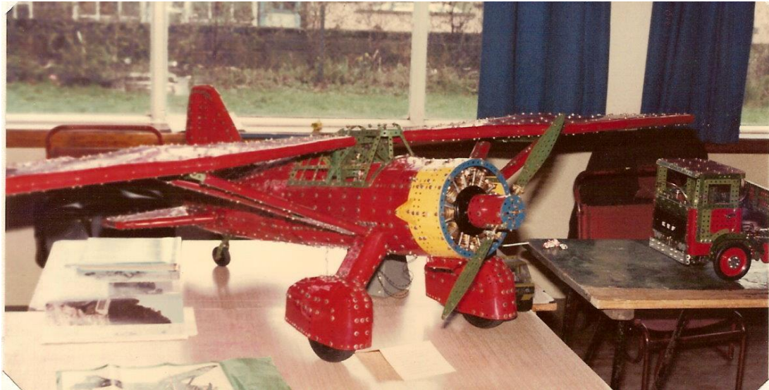
Westland Lysander Plane Built by John McDonald With a 7' wing span, moving elevators, ailerons, rudder & fitted with disc brakes and a variable pitch prop
