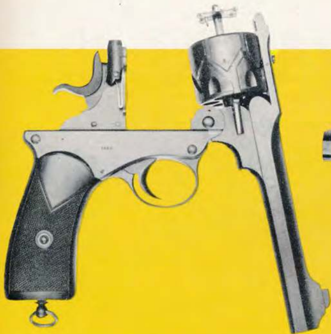
Model 1902 Webley-Fosbery revolver broken open to extract empty shells. The hammer is now at half-cock. Note quality of machining and the finish.
