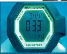
Basic diving display – current depth, elapsed dive-time and clock.
