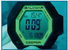
Descending below 15ft, the current depth, 15.4 ft, is shown large and the smaller 15ft preset alarm flashes and beeps. Elapsed dive time is counting up. Time is also displayed.
