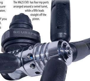
tank pressures. In the Mk25 EVO's balanced design air surrounds the piston, but doesn't act directly on it, so changes in tank pressure have almost no effect on breathing effort even when your cylinder is near empty.
