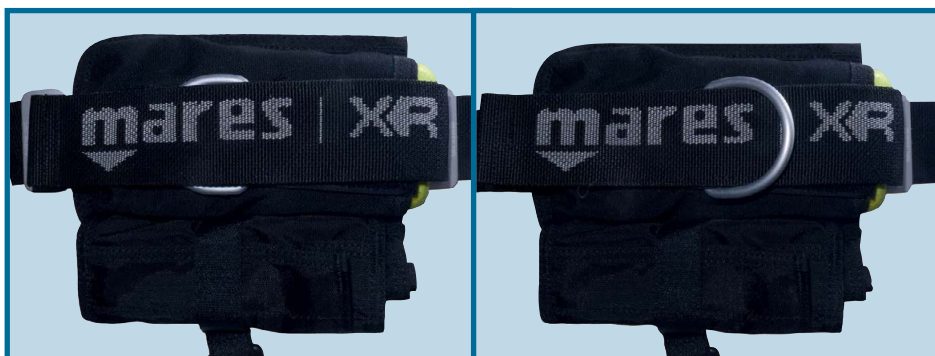
Left: Integrated weight set for fast ditching, with release-tab laid over D-ring. Right: Integrated weights set for non-ditchable diving, with strap passed through D-ring.
