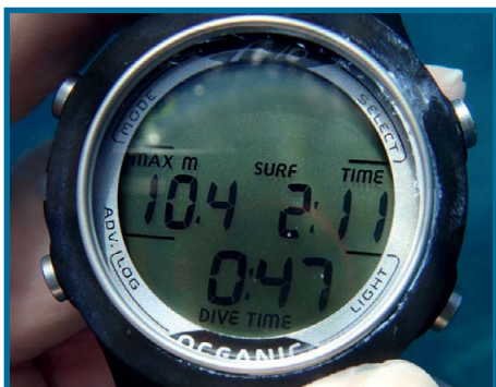
Display on surfacing, showing maximum depth, elapsed dive time, time on surface and dive number.
