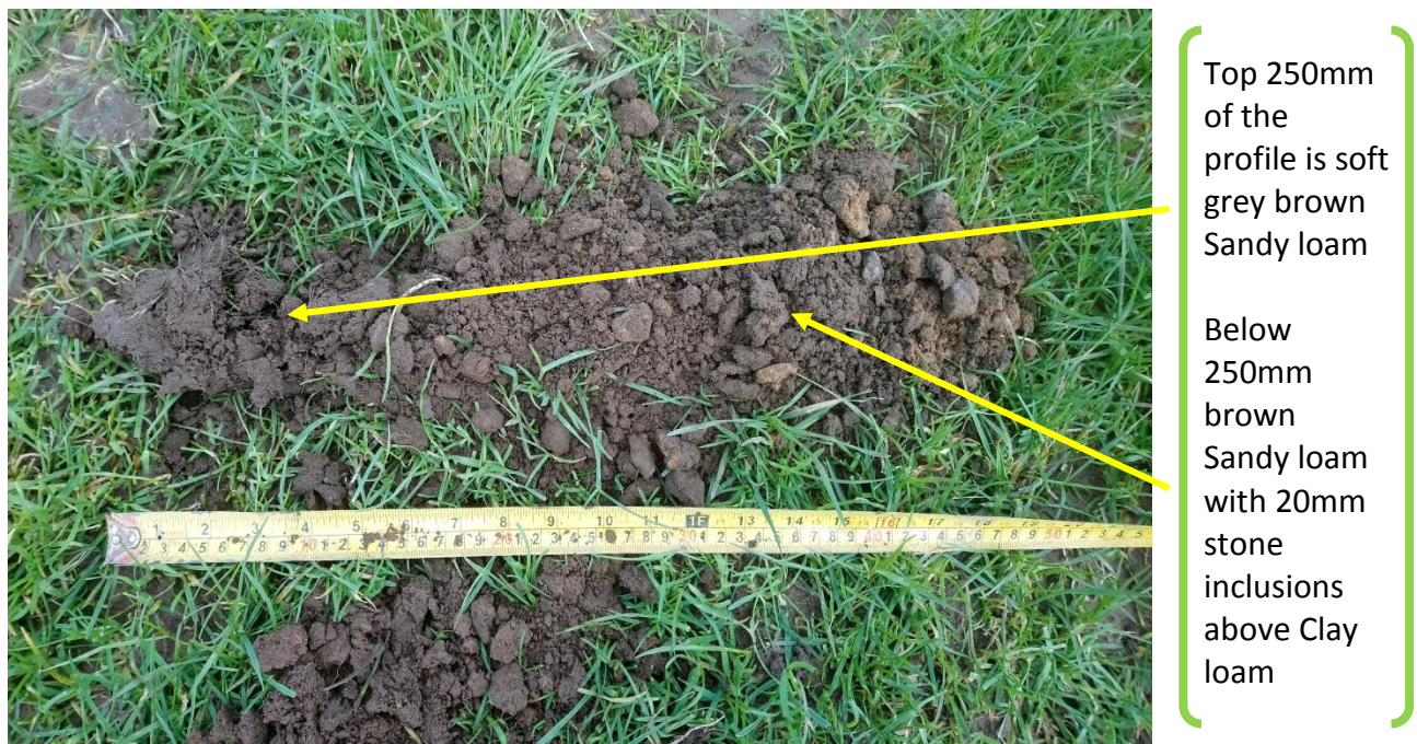
Figure 2 - Typical soil profile of the soccer pitch
