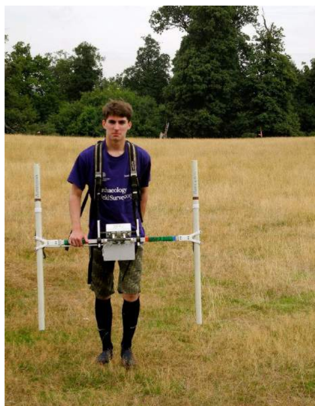
Fig. 7.10: University of Southampton student Patrick Thewlis wearing the non-magnetic clothing required for magnetometry survey. Photo by Peter Tolly.
