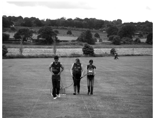
Fig. A2.11: Ivan Yeh, Emily Pierce-Goldberg and Chen Xiaowen conduct GPR survey in 2012 at the Bodiam cricket field using a 200 MHz GSSI instrument. Photo by Kathryn A Catlin.
