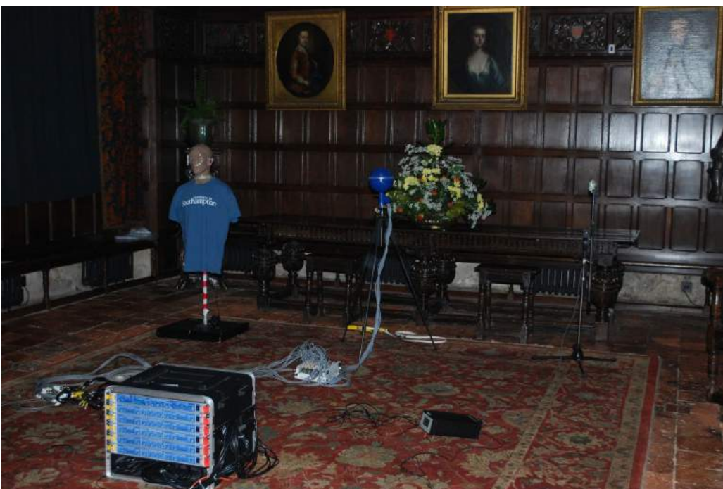
Fig. 9.17: Undertaking the acoustical survey at Ightham Mote.
