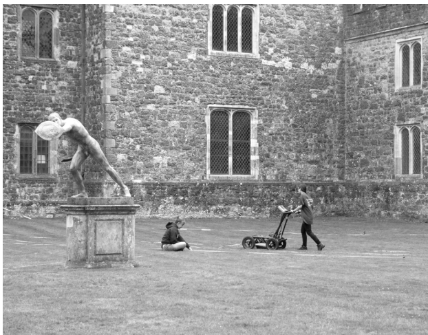
Fig. A2.10: Katie Fuller and Helena Glover conduct GPR survey in the Green Court at Knole in 2013 using a 500 MHz Sensors and Software Noggin Plus. Photo by Matthew Johnson.
