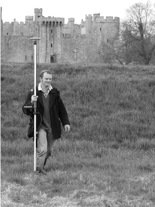
Fig. A2.1: Kristian Strutt engaged in topographic survey using RTK GPS at Bodiam Castle in 2010. Photo by Timothy Sly.
