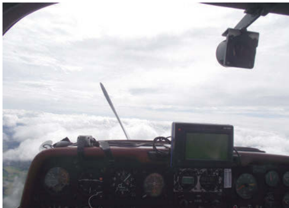
Above and below right: Grob GBXSP soaring, engine switches are off, at 6,000ft, climbing at 4m/s – propeller feathered – handle out. “They don’t ration wave lift here,” says David Innes
