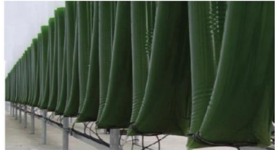
Examples of algal cultivation technologies: closed photobioreactor (Huang et al., 2017).
