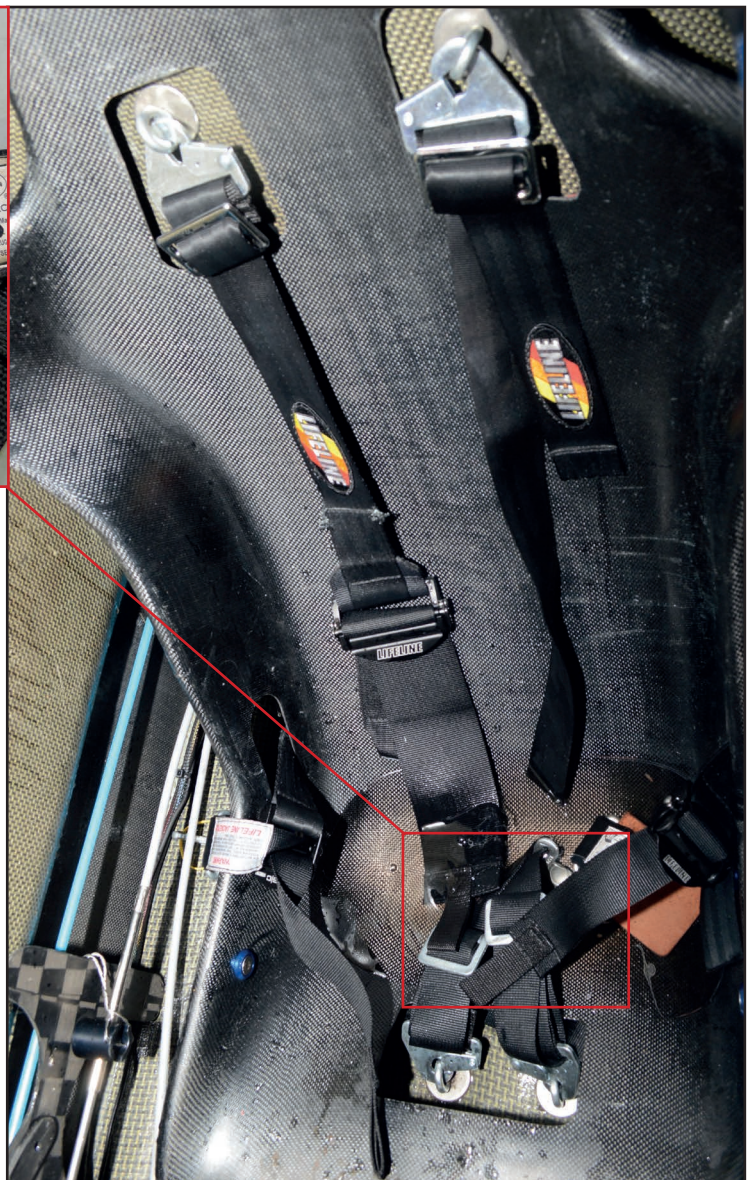
Figure 10: Boat 43 driver's harness with (inset) close-up of harness release and cable tie
