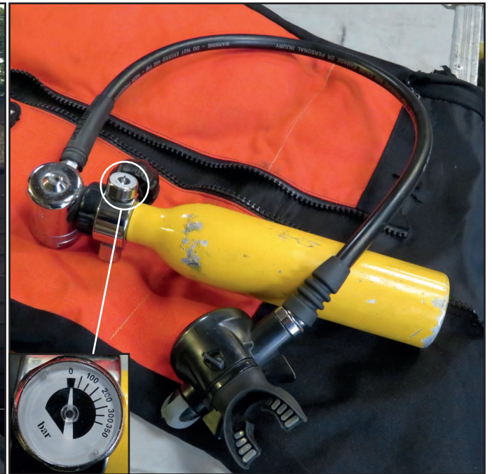
Figure 9: Boat 43's air cylinder with (inset) close-up of the air bottle gauge
