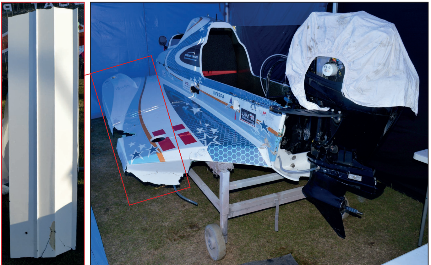
Figure 11: Boat 22 showing impact damage to port side and detached hull section
