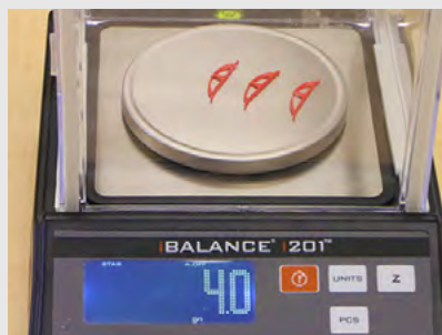
Weight of Griffin vanes with four dots of glue on each base: 4.0 grains.
