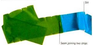
Sew the strips of ripstop together end to end to make a tail, and cut slits randomly in both sides.
