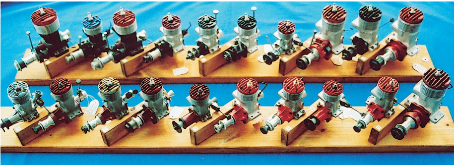
LEFT: K&B racing engines designed by Bill Wisniewski; left, the Torpedo 15R released in May 1961 for FAI C/L Speed. Right, Torpedo 29R Series 64, first released in 1961 and FAI Speed winner in '64. RIGHT: Writer's replica Ercolino 2 c.c. diesel, made by Alberto Dalloglio in Italy. The original 1942 Ercolino is said to be the first Italian-made diesel.
