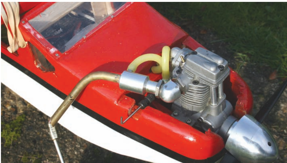
My brass tube extension, with the gentle bend formed by filling the tube with lead.
