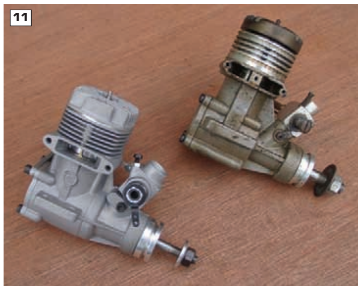
10: A digital caliper (above) is cheap and accurate enough for most work. A micrometer (below) gives more accurate readings but is limited in range. 11: Older Merco 61 (upper right) has thicker shaft than the new SC46.
