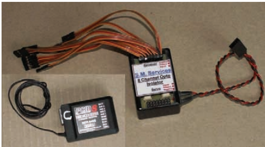
ABOVE LEFT: Connecting the servos to my JR Rx through an Opto Isolator would solve the high current problem, but I would need MatchBoxes to synchronise throw and direction of the multiple servos. ABOVE RIGHT: My preferred solution, and a very expensive one, is to use a Weatronic Dual receiver, a very large item when compared to a CD as you can see, but it should do absolutely everything required in this and future ambitious models.
