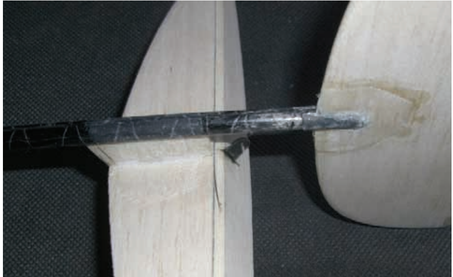
Finished back end reinforced with glass. Look in the open hinge and see the thin wire spring that keeps the elevator open. The carbon horn has a thin multi-strand wire hooked over and pulls against the spring. Simple, accurate and very light.
