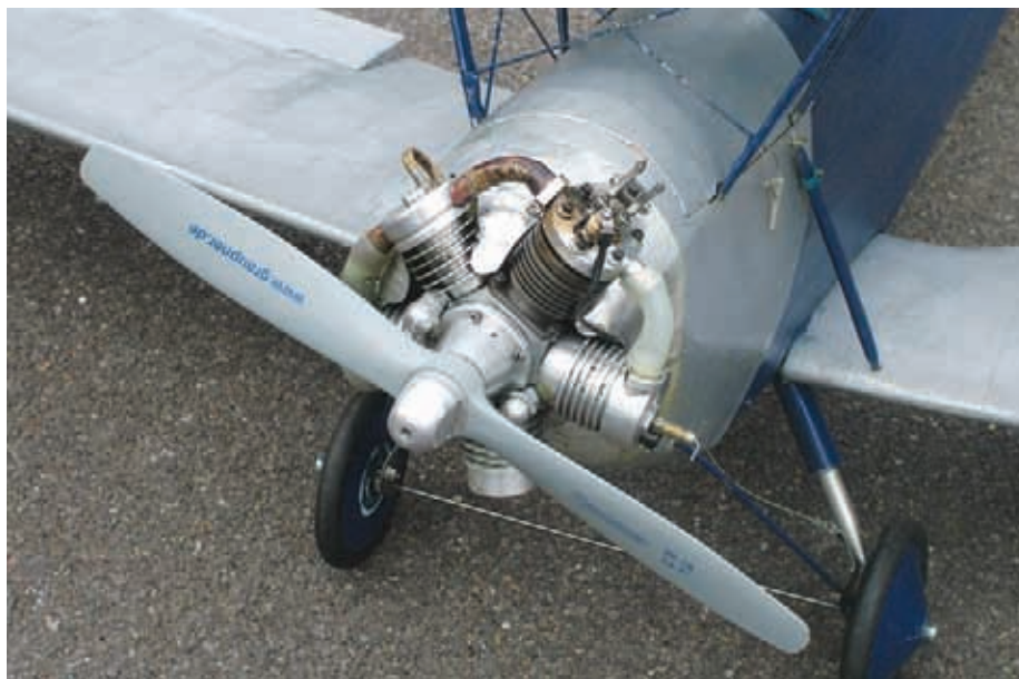
ABOVE: Chris Turner's isometric concept sketch... BELOW: ... turned into the 'five-cylinder radial'. It pulls his Hawker Tomtit around the skies with authority.
