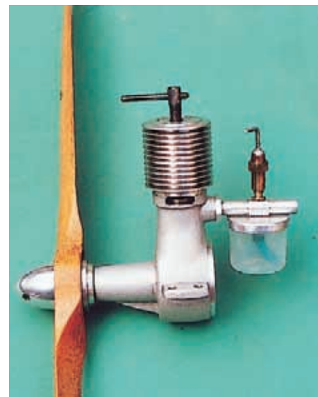
ABOVE LEFT: The little Ercolino running beautifully on an 11 x 5 Taipan composite prop. Engine exudes outstanding quality and performs well on large propellers. See text. ABOVE: C.S. (China) replica 1948 Micro 2.13 c.c. diesel; original had aluminium fuel tank but this modern version uses plastic, more practical for F/F. LEFT: The replica Micro diesel proved to be remarkably economical and enjoyed large props; here it happily turns a 14 x 4 wood at 4,300 revs. Amazing!
