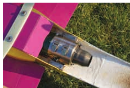
TOP LEFT: My newly added air intakes are under the wing, so here is a shot showing the air intake before the wing is attached. TOP RIGHT: Looking into the intake from in front, note the steel mesh in the fuselage side and the hole at the back that was meant to let the water go straight through. ABOVE LEFT: After suffering an instance of water ingestion, I fitted these covers over the intakes for waterplane flying. ABOVE RIGHT: I have now added this extra shield under the front of the engine which still allows plenty of air to get round to the front but will make water ingestion even less likely.
