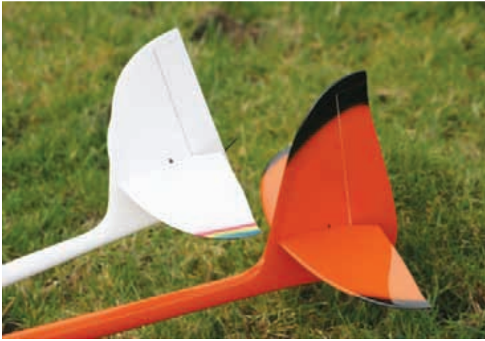
ABOVE LEFT: Compare and contrast - the Mk 1 and 2 fins are markedly different. ABOVE RIGHT: The huge fin and rudder have a lovely shape and give the Luna superb authority in yaw - very effective rudder control on this one.
