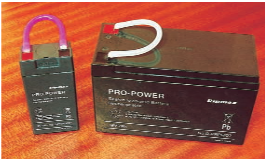
Shield and sheath your gel cell batteries' terminals with silicone fuel tube.
