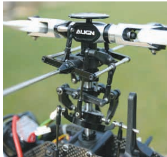
BELOW RIGHT: Close up of the completed head assembly; it's predominantly metal - ensure that threadlock is employed wherever the manual dictates.
