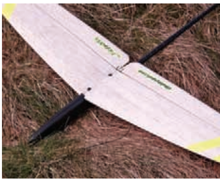
ABOVE LEFT: Ready to go and finished with logos printed on tissue and lacquer in place. ABOVE RIGHT: It's tiny at 950mm span. The tail was finished in water-soluble lacquer for lightness but some carbon tows were added to stiffen the fin and elevator. A highlighter marker adds a little trim matching those on the wing.
