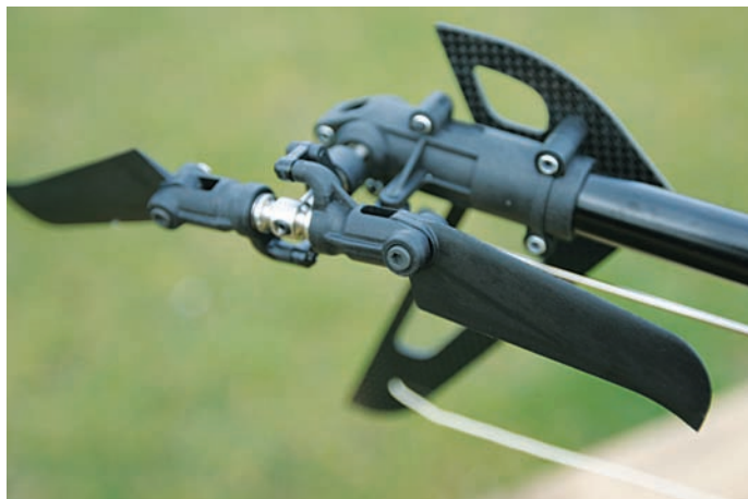
TOP LEFT: Boom-mounted tail servo mated to Futaba GY401 gyro locks the tail in. TOP RIGHT: Nice lightened 3D tailplane with boom struts supporting the boom incorporated in the mounting plate. ABOVE LEFT: Main gear installed and battery in place. All radio cabling is neatly routed and protected in conduit. ABOVE RIGHT: Tail rotor gearbox and assembly follows typical T-Rex style and design with toothed belt drive within the boom.
