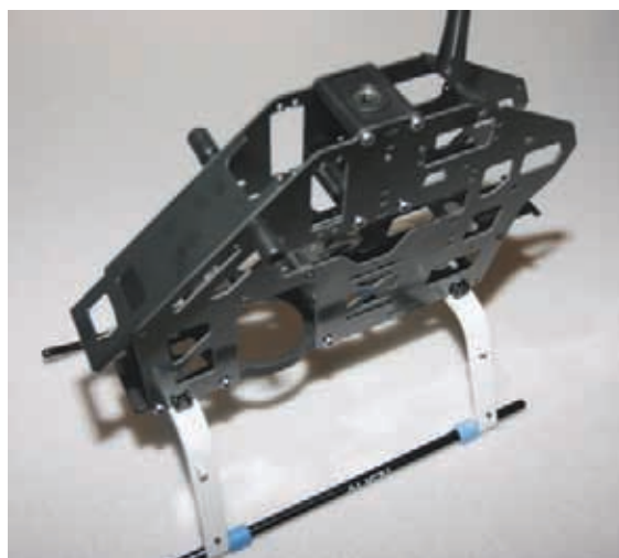
The addition of an undercarriage makes for a stable building platform.
