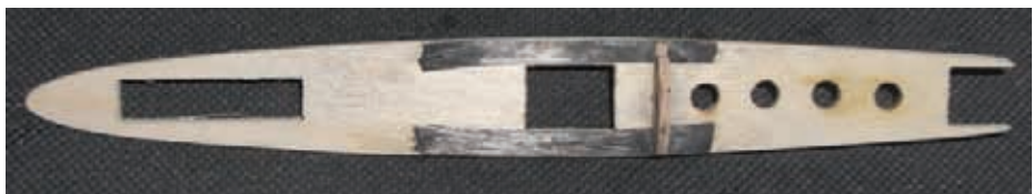
Modified with a former, which wasn't part of the instructions. The lightening holes gave about the same amount of wood removed as that added!
