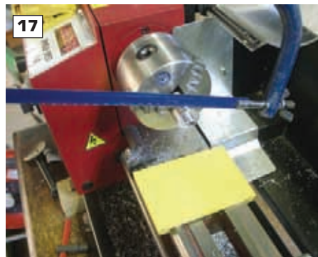
14: After drilling 15/64in. the final step is to run in the 1/4in. drill. 15: A series of cuts is taken to reduce the diameter. 16: The Vee tool is employed to cut a groove. 17: 'Parting off' with a hacksaw. 18: Sawn surface is still visible, prior to a facing cut.
