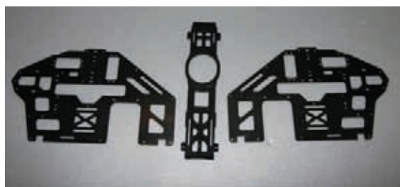
Handed carbon side frames and base moulding form the basis of construction.
