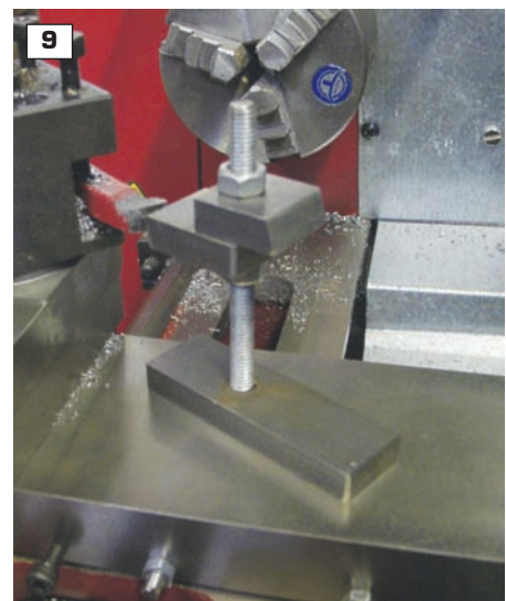
ABOVE: Drive is taken by a train of gears from the spindle (top) down to the lead screw (lower right). The tumbler arrangement provides a feed reversal facility, useful for left hand threads. BELOW: This easily made gauge speeds up tool height setting.
