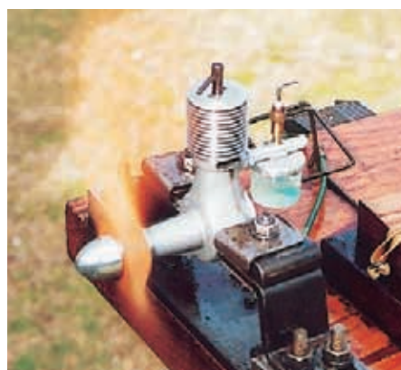
ABOVE LEFT: The little Ercolino running beautifully on an 11 x 5 Taipan composite prop. Engine exudes outstanding quality and performs well on large propellers. See text. ABOVE: C.S. (China) replica 1948 Micro 2.13 c.c. diesel; original had aluminium fuel tank but this modern version uses plastic, more practical for F/F. LEFT: The replica Micro diesel proved to be remarkably economical and enjoyed large props; here it happily turns a 14 x 4 wood at 4,300 revs. Amazing!
