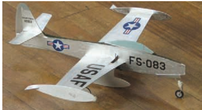
This profile model of the Beavors' Republic F-84 Thunderjet uses a cunningly disguised propeller rotating in a slot in the fuselage. The pair of large, low-slung bombs (or are they fuel tanks?) probably also help to keep fingers away from the blades. This model beautifully illustrates the pleasure of simple RTP models.
