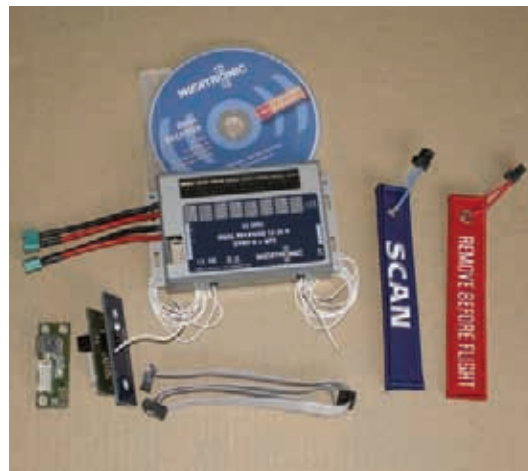
ABOVE LEFT: Connecting the servos to my JR Rx through an Opto Isolator would solve the high current problem, but I would need MatchBoxes to synchronise throw and direction of the multiple servos. ABOVE RIGHT: My preferred solution, and a very expensive one, is to use a Weatronic Dual receiver, a very large item when compared to a CD as you can see, but it should do absolutely everything required in this and future ambitious models.
