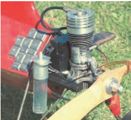
All kind of engine modifications are permitted in the TEXACO class. Here is home made cylinder head for a Super Cyclone ignition engine.
