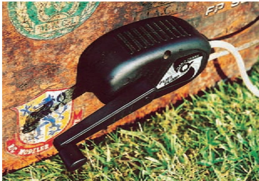
BELOW LEFT: Gerard's thirty-year-old flight box may look rough (like himself!) but it still proves to be ultra-reliable. BELOW RIGHT: Gerard really approves of the hand-cranked fuel pump he has fitted to his downmarket flight box. If you want hassle-free fuel tank filling and emptying, get one of these items now!
