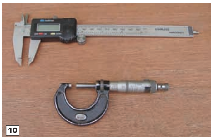
10: A digital caliper (above) is cheap and accurate enough for most work. A micrometer (below) gives more accurate readings but is limited in range. 11: Older Merco 61 (upper right) has thicker shaft than the new SC46.
