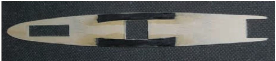
Standard liteply radio tongue, reinforced with carbon tows using thin cyano.
