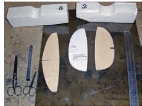
LEFT: As it comes - tiny and doesn't seem very much for your money! ABOVE: Prepare first and make sanding blocks and templates for sanding the section in the fin and tailplane. A piece of glass makes an excellent flat surface to work on.
