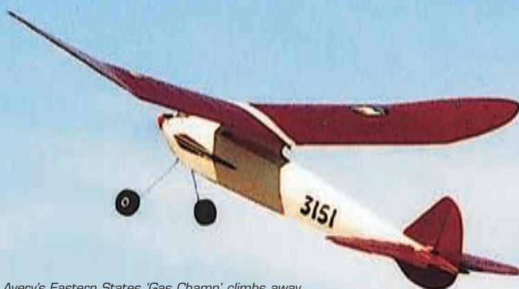
Ian Avery's Eastern States 'Gas Champ' climbs away in a Duration event at 2006 Oz Nats at Loxton, S.A. Engine is an O.S. 32 two-stroke heli glow.
