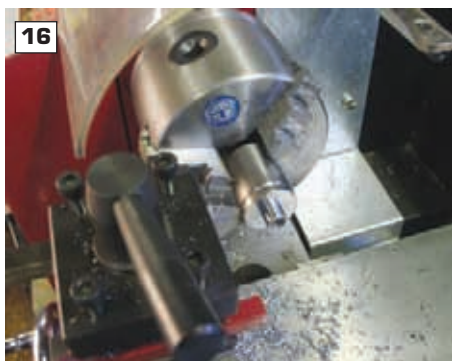
14: After drilling 15/64in. the final step is to run in the 1/4in. drill. 15: A series of cuts is taken to reduce the diameter. 16: The Vee tool is employed to cut a groove. 17: 'Parting off' with a hacksaw. 18: Sawn surface is still visible, prior to a facing cut.
