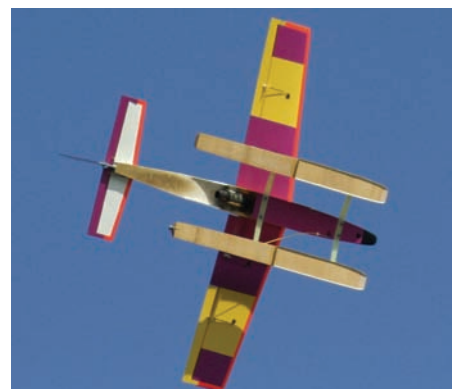
TOP LEFT: The early jet trainer models like this Kangaroo had the engine mounted up on top of the wing, fully exposed. TOP RIGHT: John Agnew's Fox Cub jet trainer with a Wren 44 hanging out in the open - but you never see full-size aircraft like this. ABOVE LEFT: On my model I tried to hide the engine away but still have it easy to mount and to work on. ABOVE RIGHT: In this shot of the underside you can see that the engine is fully accessible from below, and you can also see that there are no intakes on the fuselage sides. The air gets to the engine from below. Note also the burnt oil marks on the ceramic blanket covering the underside.
