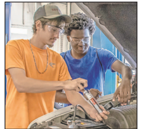
Austin Kortzendorf and Mayki Jones checking radiator pressure.
