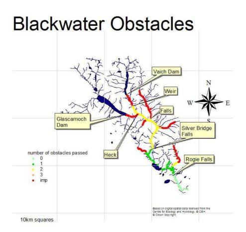
The fish ladder at Rogie is well designed and allows fish to ascend at a wide range of flows. However in very low flows Rogie Falls can delay migrating salmon and the pools downstream are especially vulnerable to poaching. Glascarnoch and Vaich Dams have no provision for fish passage and cut off the headwaters of the system. A weir constructed in Strath Vaich restricts trout movement but also modifies habitats upstream and could be removed as it no longer fulfils a function.
