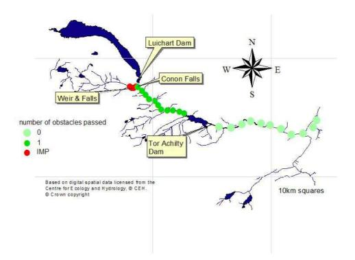
The lowest significant obstacle in the Conon is Tor Achilty Dam. Tor Achilty has a Borland lift to provide fish passage. The main impact on adult fish is an increase in predation, particularly by otters, when fish are delayed and congregate below the dam. Smolts passing downstream are vulnerable to avian and fish predators, either when delayed above the dam or disorientated after passing through the turbines. Migrating silver eels are at risk of damage when passing through the turbines.
