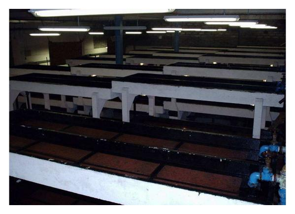
The Contin Hatchery contains 32 troughs each with three tiers and a separate water supply. There are also 8 2m tanks used for first feeding salmon fry. The total capacity of the Contin Hatchery is 4 million ova.
