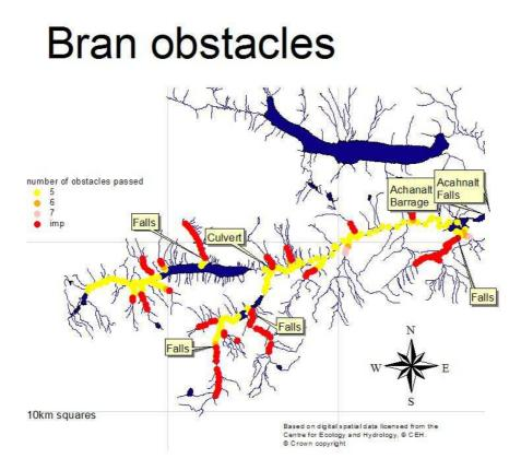
The fish ladder at Achanalt was modified as a result of radio-tracking work to improve its performance. There is still an increased risk of predation by otters and of poaching below the ladder. The small Borland Lift in the centre of Achanalt Barrage may allow some fish to pass upstream but it is equally likely that fish will pass under the Barrage gates which are opened even after moderate rainfall.
